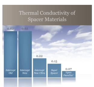
The lower the thermal conductivity, the warmer the glass—and the more comfortable you feel. Vytex DuraTex<sup>TM</sup> Warm Edge Spacer System offers a 50% improvement in thermal conductivity over Super Spacer and an 80% improvement over Intercept.
